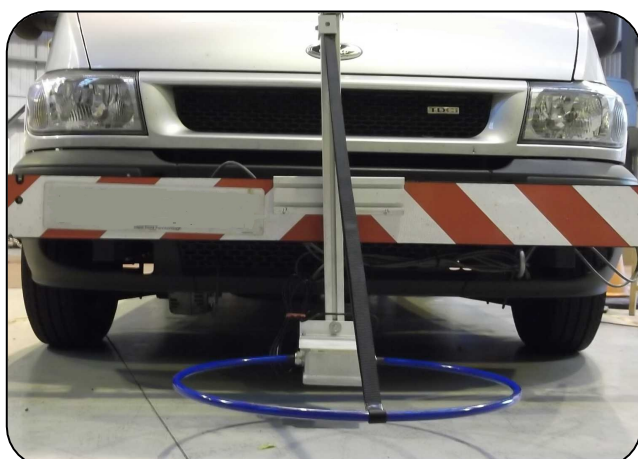
Figure 8 – Survey vehicle with front mounted RFID antenna
